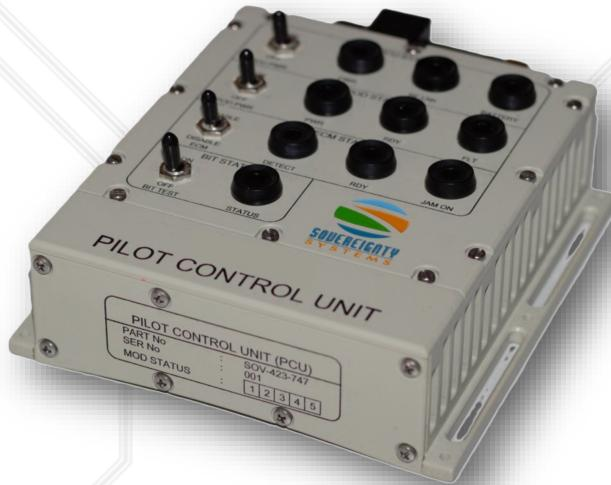
The PCU System is a wireless control and communication system designed to provide the pilot with remote control & monitoring of various equipment that is otherwise external to the aircraft.
